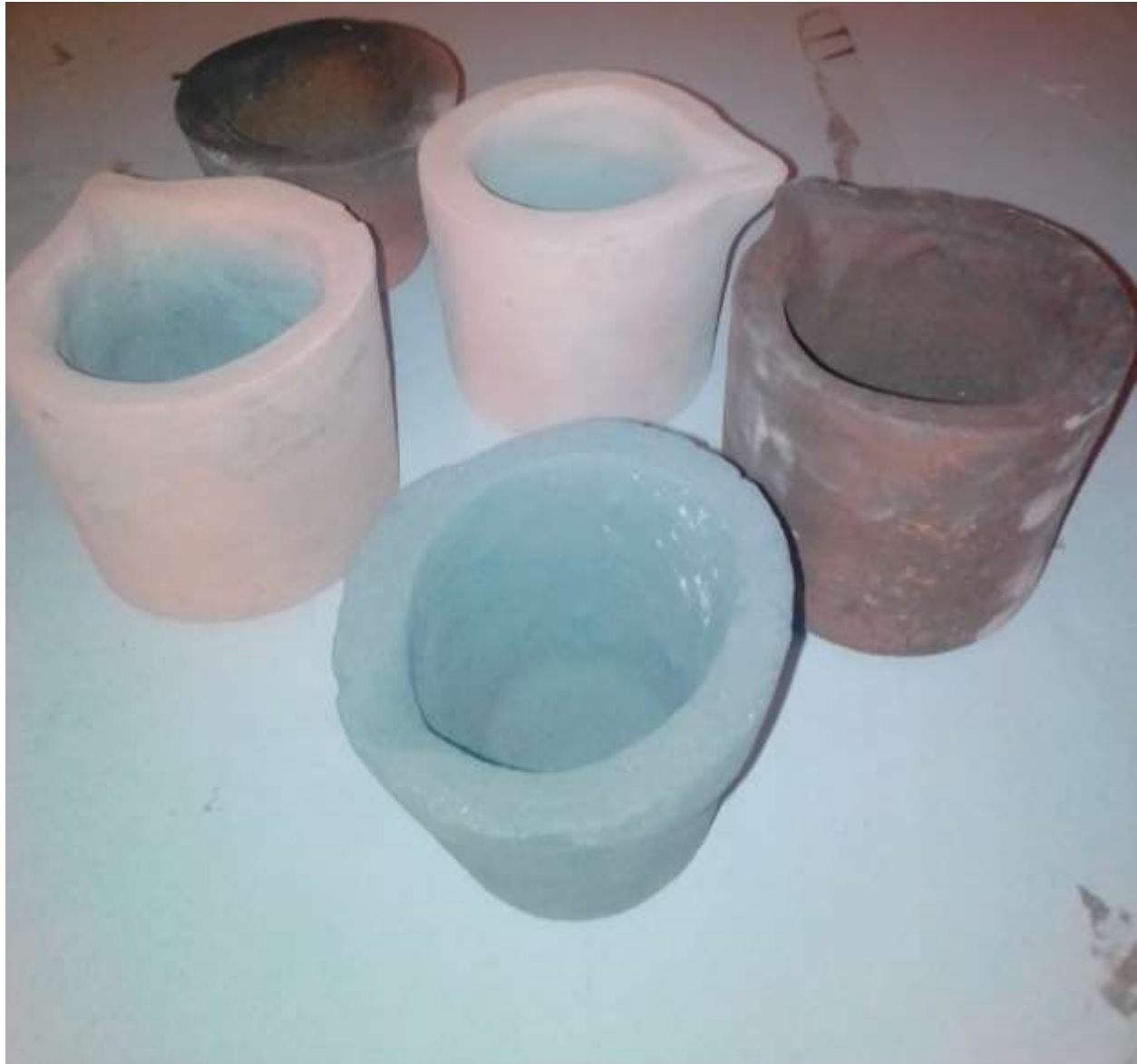
Plate XV: Graphite crucibles produced
