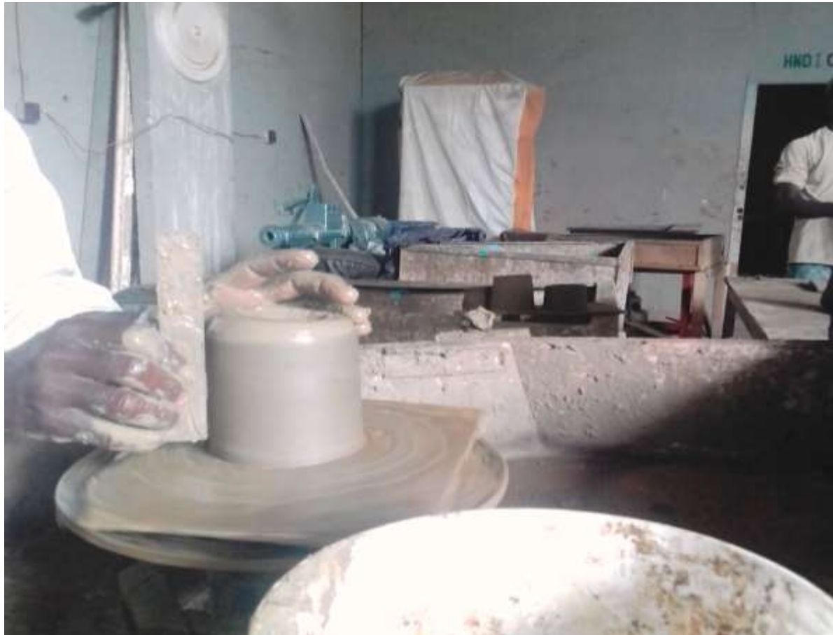
Plate XII: A model of crucible being produced for slip casting
